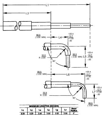
Customer to specify L4 & L5 or L6 & L7. L1 & L2 are specified in Model number.
